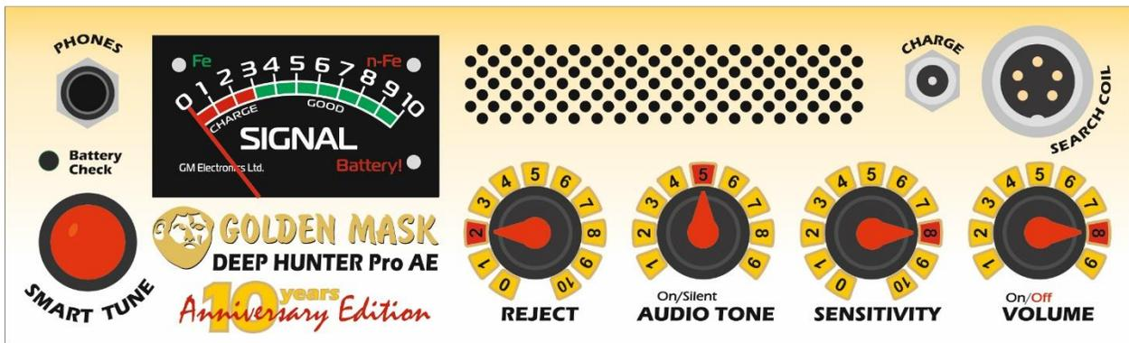
“**VOLUME On/Off**” - knob to switch “ON/Off” the detector and adjusting the level of sound.
